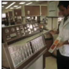
QUV accelerated weathering testing device.
